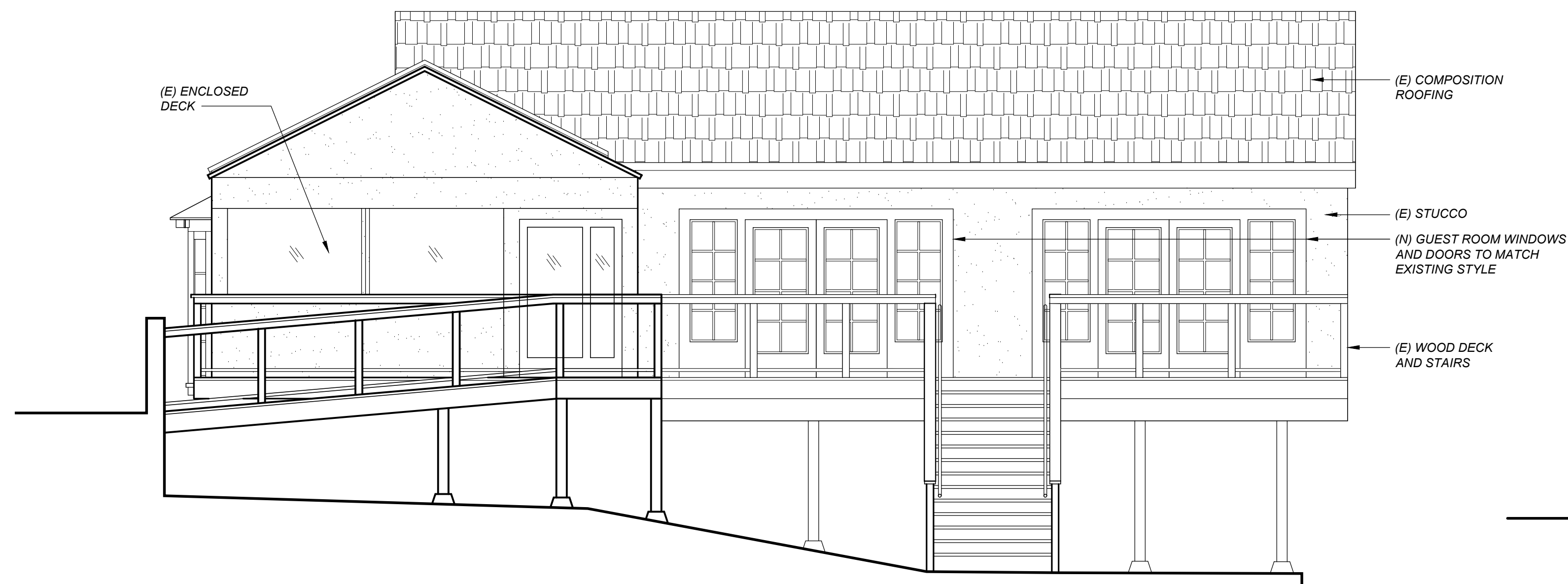
MODIFIED DOORS AND WINDOWS OF NORTH ELEVATION
