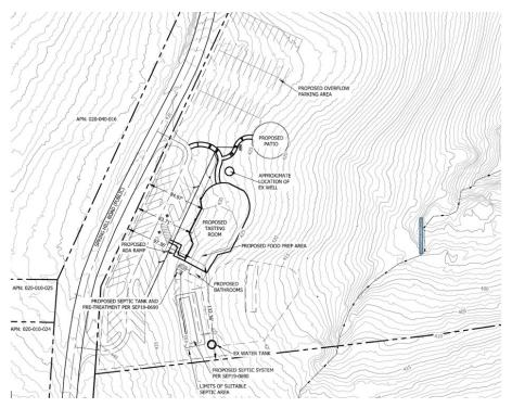
Figure 6: Close up of Proposed Tasting Room and Associated Improvements
