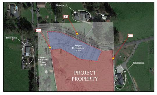
Figure 12: Project Site Development Area, Surrounding Uses and Noise Measurement Locations
