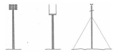
The silhouette is a calculation of the physical surfaces of the combined tower and antenna(s) included in a telecommunication facility. Only the physical surfaces, and not the air spaces in between, are counted in the calculation. The silhouette calculation is measured from the viewing angle which presents the largest exposure from an elevation perspective.
