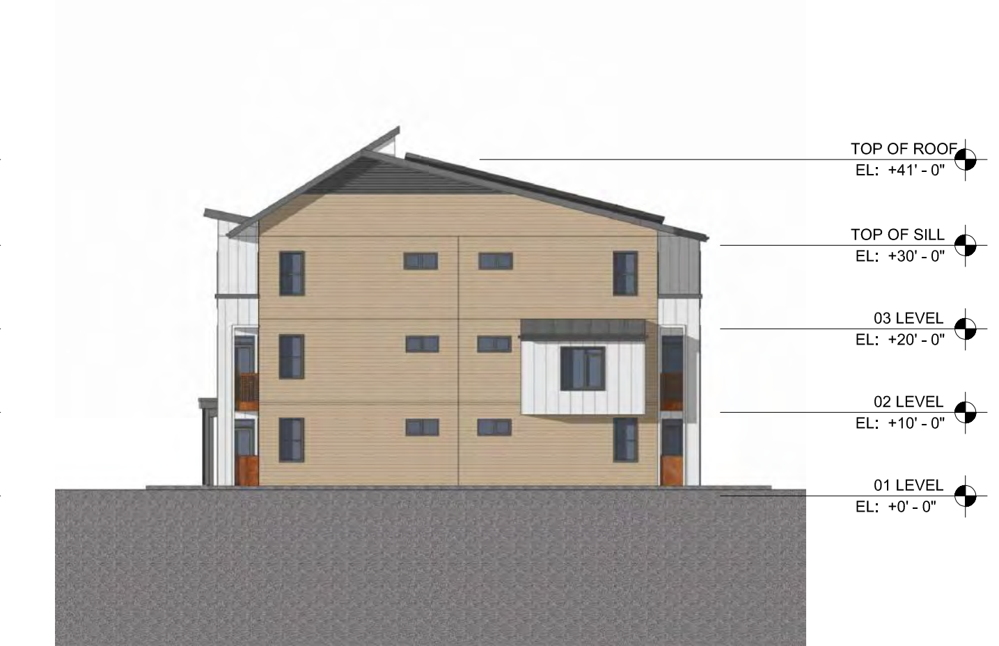
C2 BUILDING- LEFT ELEVATION
