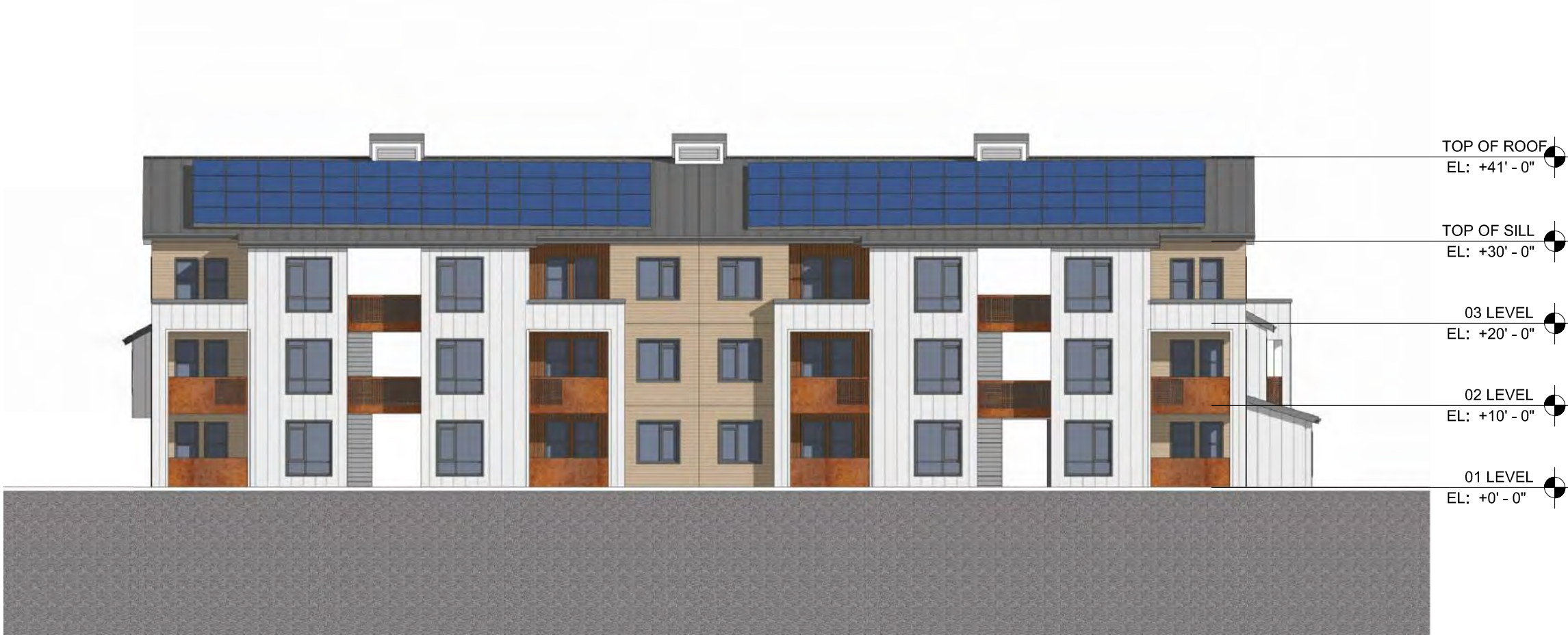
C2 BUILDING- FRONT ELEVATION
