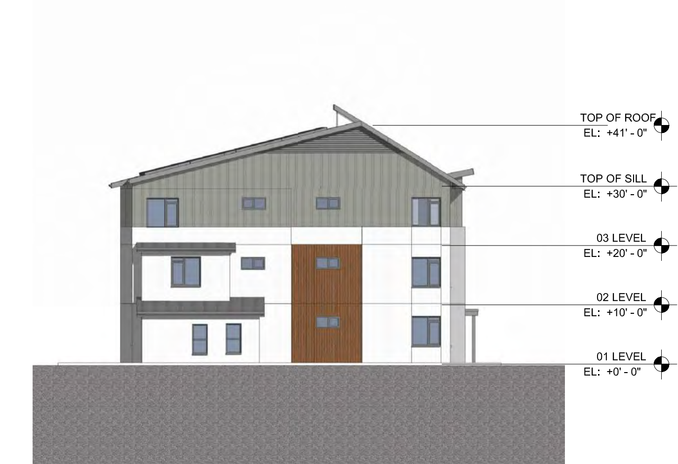
C3 BUILDING- RIGHT ELEVATION
