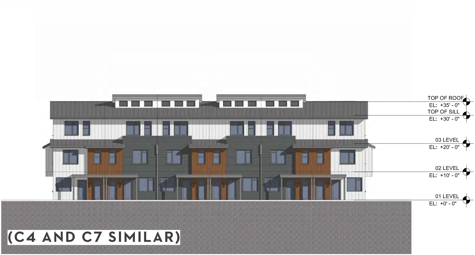
C1 BUILDING- FRONT ELEVATION
