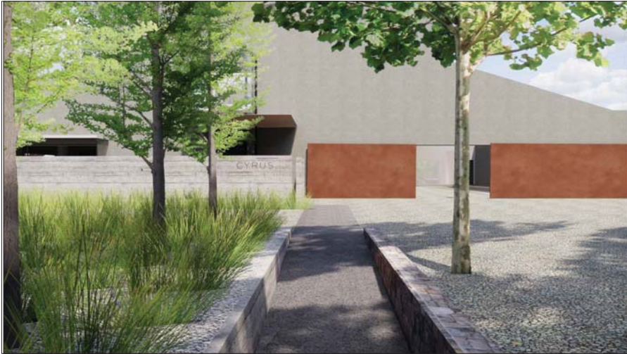
VIEW FROM PROPOSED SLOPED PATH - PROPOSED GREY BOARD FORM CONCRETE WALL AND RUSTED STEEL CLADDING ON BUILDING
