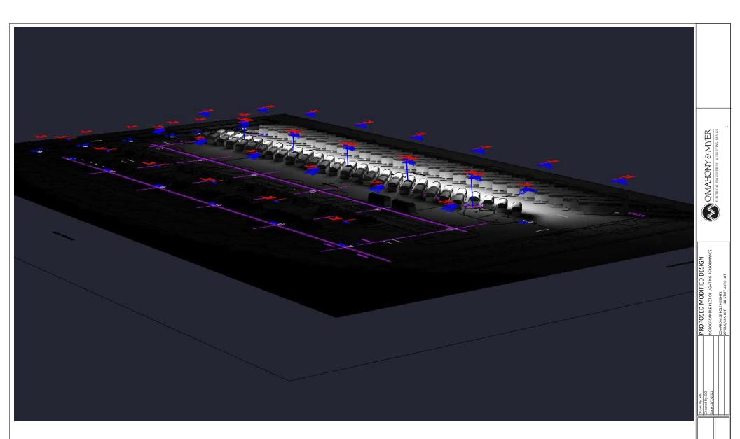
Computer Rendering of Compromise Scheme w/ SECURITY LIGHTING SYSTEM LUMINAIRES ONLY TURNED 'ON'
